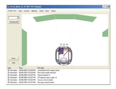
**Distance** – Used to move the robot set distances and rotate set degrees
