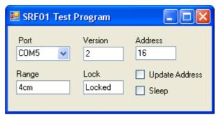
We have a small test program, written in C# which controls the SRF01 via the <u>Acroname S22</u> module. A small schottky diode is used to prevent the SRF01 trying to drive the S22's output line (data from the PC). You will need to download and install the <u>FTDI VCP</u> drivers to use the S22.
