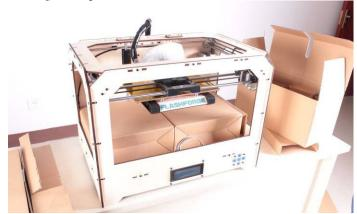
Now you should be able to see underneath the build platform, you'll find the filament here; either one or two rolls, depending on whether your Creator has one or two extruders. It's easiest to remove the filament by setting aside the remaining packaging material.
