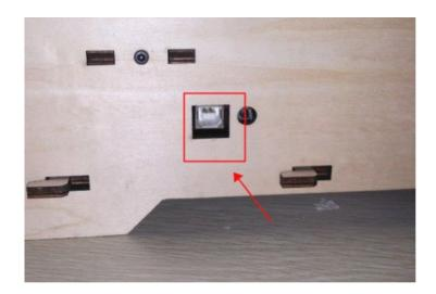
The USB port on the machine is bound by the red box in the above image. After connecting the cable, open the Replicator G software, we are going to connect the computer and printer.
