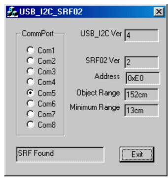
Connecting the SRF02 to your PC via USB is this easy. The USBI2C module supplies the SRF02 with power directly from the USB bus. The USB\_I2C\_SRF02 program can be <u>downloaded here</u>.
